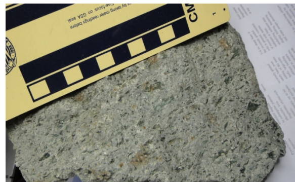
Figure 4. Preferential alteration of pumice/fiamme to chlorite-sericite gives a “Swiss cheese” feature.
