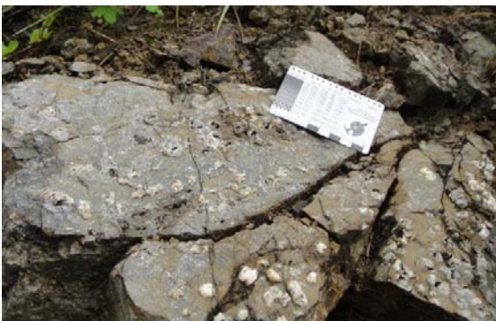
Figure 5. Devitrification zone with abundant spherulite/lithophysae in welded ignimbrite.
