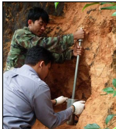
Figure 3. KU - miniature sampler (Mairaing et al., 2005).
