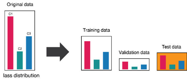
Figure 2 A diagram shows stratified sampling where the data are split while class distribution remains constant.
