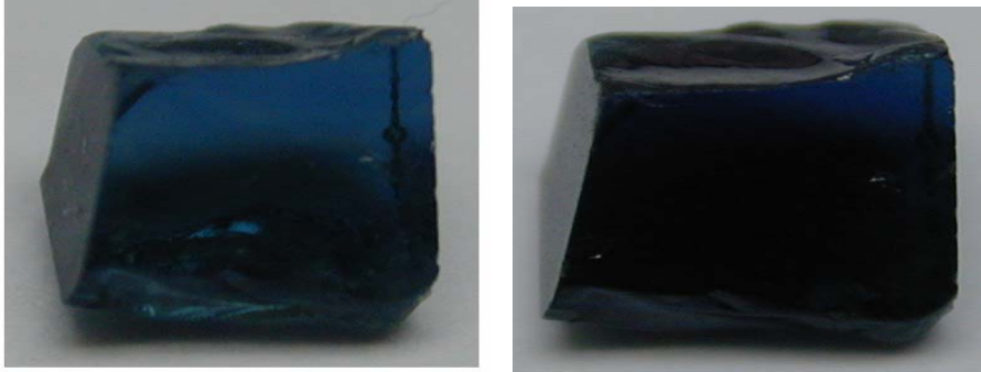
Figure 26: Showing the color appearance in a blue sapphire (APLB8) before (left) and after heating (right).
